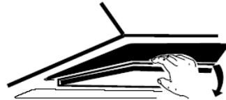
Plug the activated carbon filter into the unit and turn it in clockwise direction. Repeat the same on the other side.
